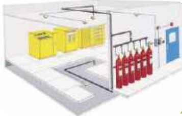
GAS BASED SUPPRESSION SYSTEM
